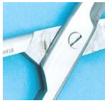
Joint showing wear due to inadequate lubrication
