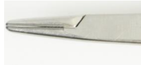
Needle-holder with damaged jaw
